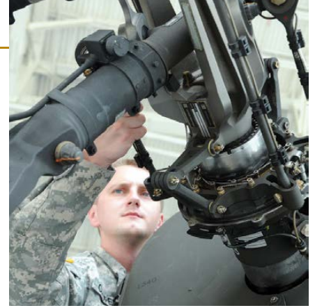
A member of the Mississippi Army National Guard inspects the rear rotor of an AH-64 Apache during daily maintenance at the Combat Readiness Training Center in Gulfport, Mississippi. (Photo: Mississippi National Guard)
